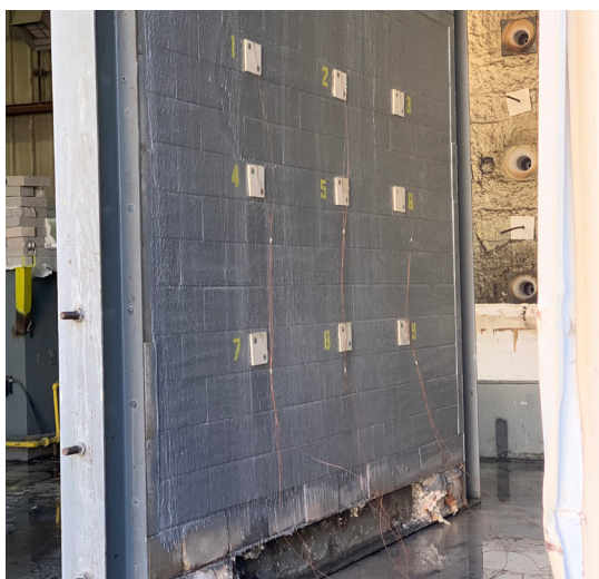
Exposed side of SC-3900-coated block wall post stream test with no water pass-through.
