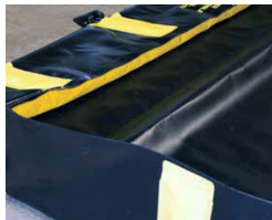
Fail-Safe® flotation device on both the entry and exit walls is self-erecting and will rise as the fluid level rises. The entry/exit walls also have the brace support, which will lock into position with the rising fluid level.
